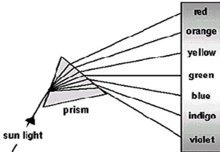
**When white light, such as sunlight passes through a prism, it is refracted in the colors of the rainbow.**
